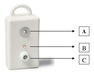
Plug in the 1.5 mm connector of lead wire, gold cup or jumper cable into plug in on wire tester – on diagram above marked as "C". Snap on lead wire or place gold cup on metal button area on wire tester – on diagram above marked as "A". With jumper cables, place the plug in containing a gold post onto button area. The light will come on (area marked "B") if a continuous current is detected.
